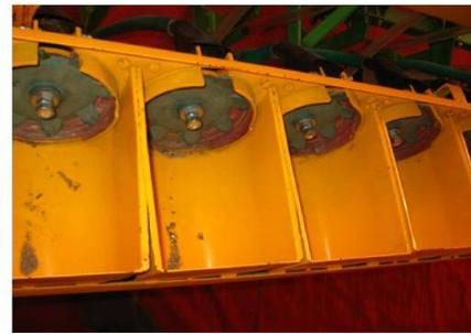
Fig.1 (b) Metering mechanism
