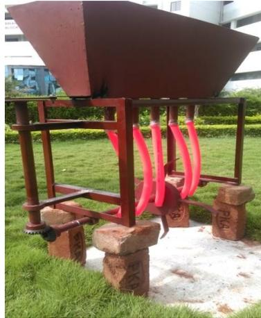
**Fig.6.1 Proposed sowing machine**
