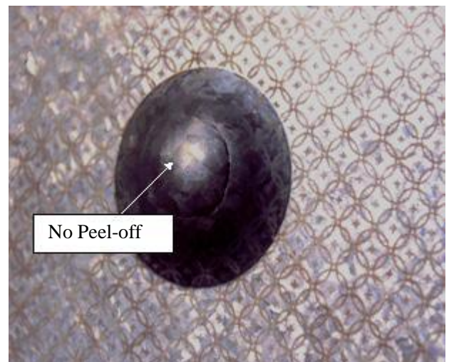
Figure 7. Strain analysis in formed component of (a) Conventional GI sheet (b) Zn-Mg coated sheet
