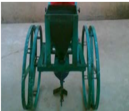
Plate III: The Developed Manually Operated Single-Row Multi-Crop Planter
