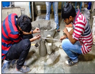
Figure 5: Slump measuring during concrete trails.
