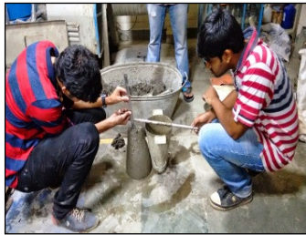
Figure 5: Slump measuring during concrete trails.
