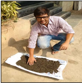
Figure 3 Drying of River sand before sieve analysis.
