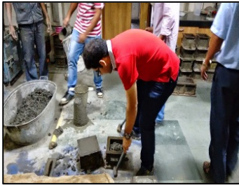
Figure 4 : Compacting cube using rubber hammer &
