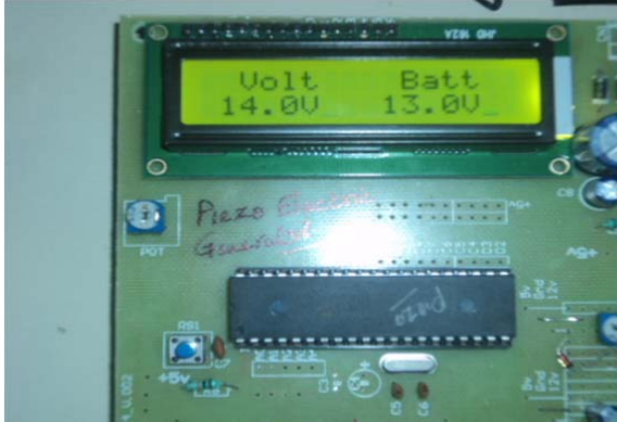
Figure.3 Showing the piezo electric generator IC89C52 Microcontroller displaying output of our work
