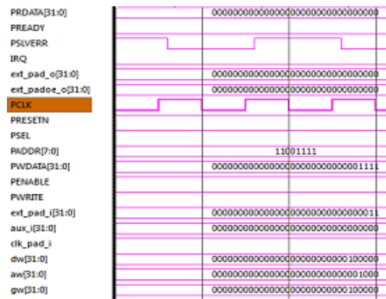
Figure 6. Simulation result of PSLVERR (Failure)
