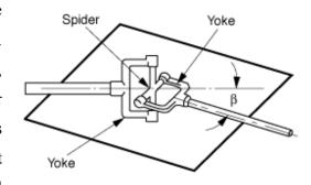
design practice calls for low operating angles, often less than 25°, depending on the application. Independent of this guideline ne, mechanical interference in the construction of Cardan joints limits the operating angle to a maximum (often about 37½°), depending on its proportions. Typical applications of universal joints include aircraft, appliances, control mechanisms,
