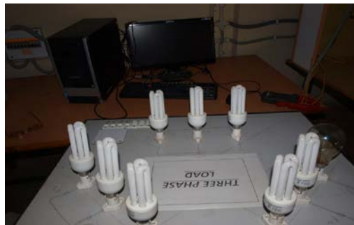
Figure (12) C.F.L Load Experimental Setup for CFL
