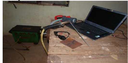
Figure 4 Single phase ARC welding machine setup
