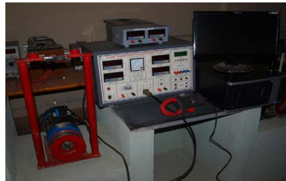
Figure 9 D.C. Motor Drives experimental set-up
