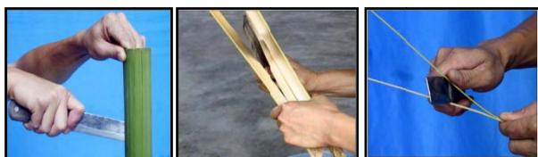
Fig. 10 Traditional/old Methods of making splits and Slivers from bamboo by hands
