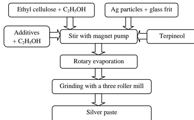
**Fig-2:** Flow sheet for preparing silver front contact paste
