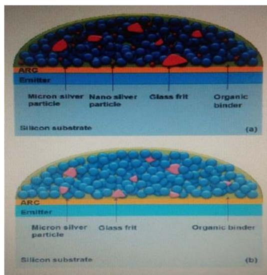
**Fig-3:** Schematic diagrams of the printed silver fingers before firing treatment: (a) Containing hybrid of micron
