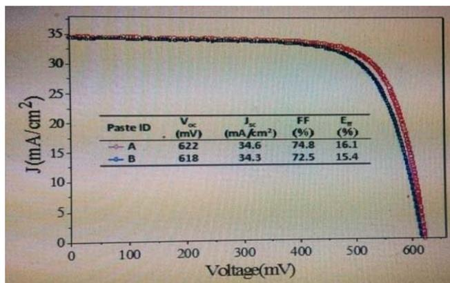
**Fig-5:** I-V performance of the fabricated crystalline silicon solar cells based on different silver pastes under AM 1.5 (1000W/m<sup>2</sup>).
