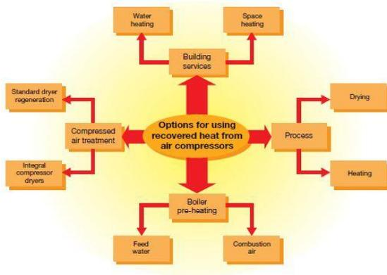
Fig.3. Heat Recovery with Rotary Screw Compressors [1]
