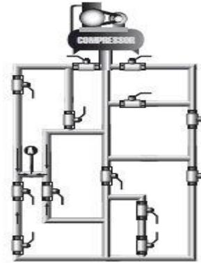
Fig.5. closed loop network
