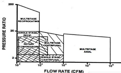
Fig.2.Compression between the different types of compressor[5]
